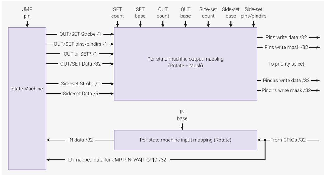
The write data and write masks for the output level and output enable registers come from the following sources:
