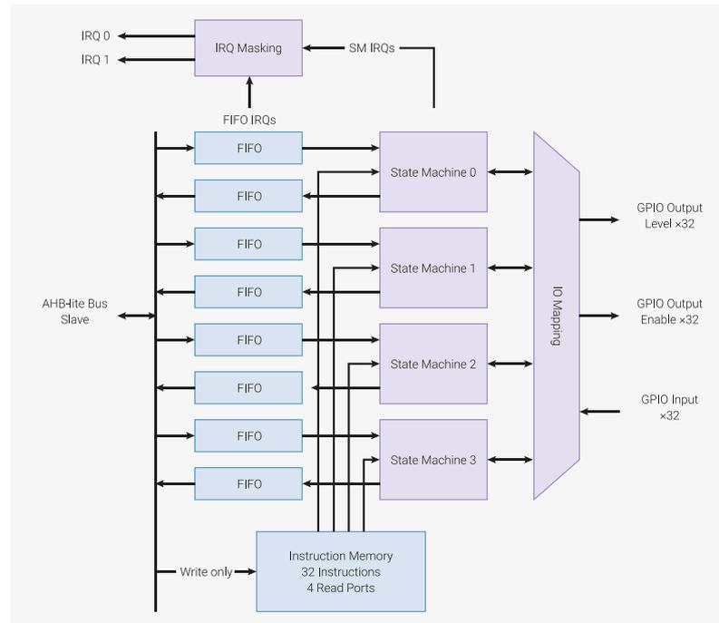
The programmable input/output block (PIO) is a versatile hardware interface. It can support a variety of IO standards, including:
