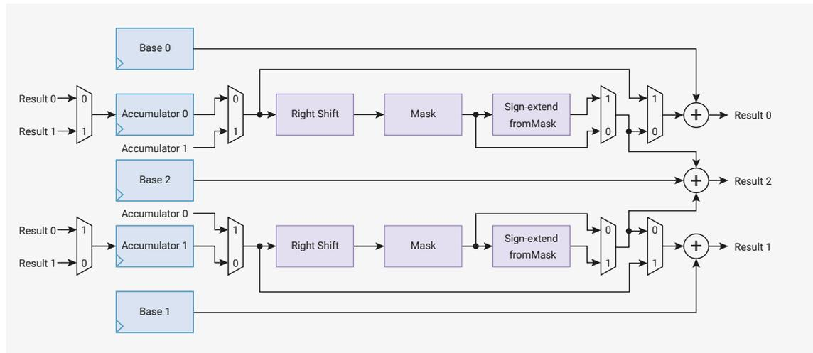
The processor can write or read any interpolator register in one cycle, and the results are ready on the next cycle. The processor can also perform an addition on one of the two accumulators **ACCUM0** or **ACCUM1** by writing to the corresponding **ACCUMx\_ADD** register.
