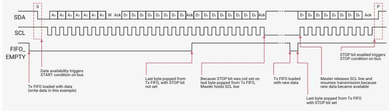
Figure 74 illustrates the behaviour of the DW\_apb\_i2c when the Tx FIFO becomes empty while operating as a master receiver, as well as showing the generation of a STOP condition.
