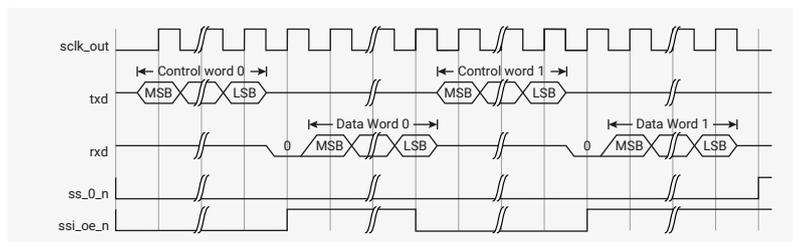
The only modification needed to perform a continuous nonsequential transfer is to write more control words into the transmit FIFO buffer; this is illustrated in Figure 137. In this example, two data words are read from the external serial-slave device.
