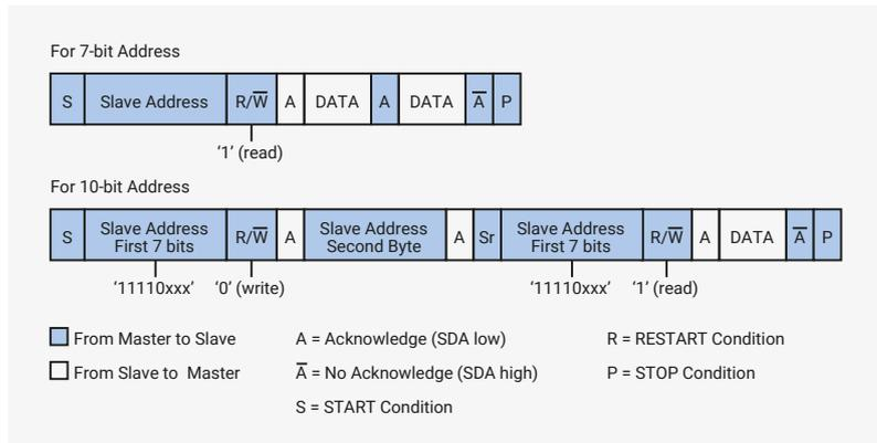
When a master does not want to relinquish the bus with a STOP condition, the master can issue a RESTART condition. This is identical to a START condition except it occurs after the ACK pulse. Operating in master mode, the DW\_apb\_i2c can then communicate with the same slave using a transfer of a different direction. For a description of the combined format transactions that the DW\_apb\_i2c supports, refer to Section 4.3.5.2.
