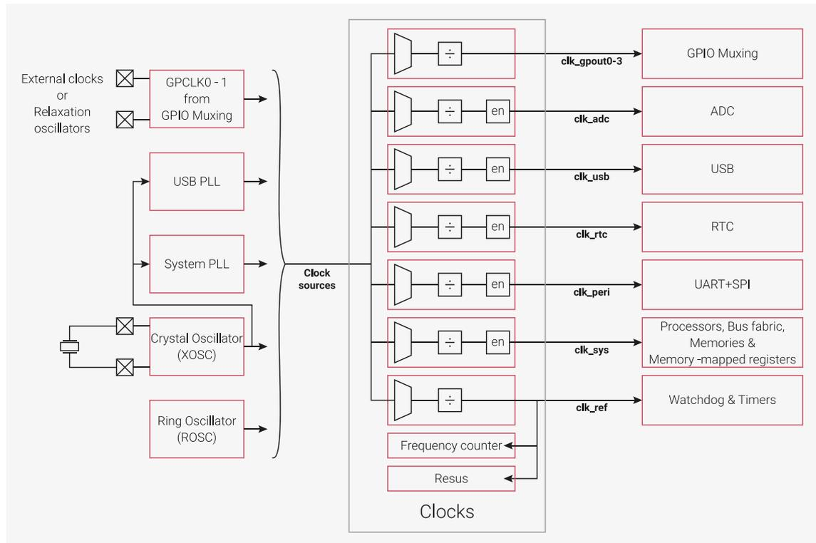
For very low cost or low power applications where precise timing is not required, the chip can be run from the internal Ring Oscillator (ROSC). Alternatively the user can provide external clocks or construct simple relaxation oscillators using the GPIOs and appropriate external passive components. Where timing is more critical, the Crystal Oscillator (XOSC) can provide an accurate reference to the 2 on-chip PLLs to provide fast clocking at precise frequencies.
