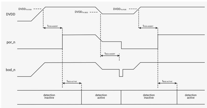
Once the chip is out of reset, detection can be disabled under software control. This also saves a small amount of power. If detection is subsequently re-enabled, there will be another short delay, the *brown-out detection enable delay* (t<sub>BOD.ENABLE</sub>), before it becomes active again. This is shown in Figure 25.
