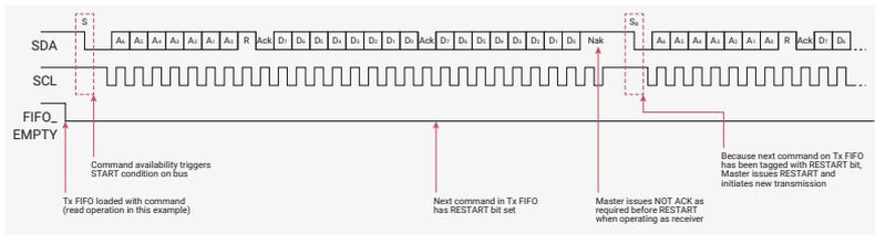
Figure 77 illustrates operation as a master transmitter where the Stop bit of the IC\_DATA\_CMD register is set and the Tx FIFO is not empty
