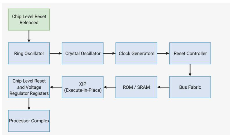
The power-on state machine sequence is as follows:
