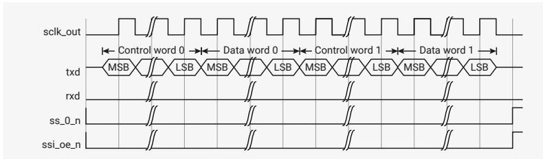
The only modification you need to make to perform a continuous transfer is to write more control and data words into the transmit FIFO buffer, shown in Figure 143. This example shows two data words are written to the external serial slave device.
