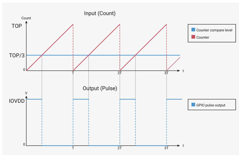
This example shows the counting period and the A and B counter compare levels being configured on one of RP2040's PWM slices.
