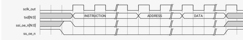
To initiate a Dual/Quad write operation, CTRLR0.SPI\_FRF must be set to 01/10/11, respectively. This will set the transfer type, and for each write command, data will be transferred in the format specified in CTRLR0.SPI\_FRF field.
