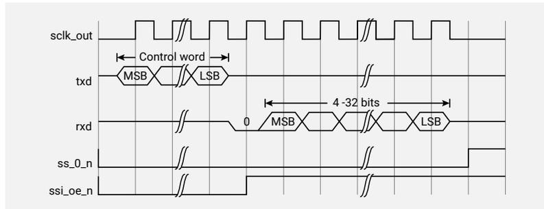
Figure 135 shows how the data and control frames are structured in the transmit FIFO prior to the transfer; the value programmed into the MWCR register is also shown.
