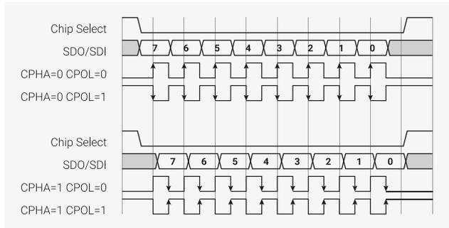
SPI is a common serial interface with a twisty history. The following program implements full-duplex (i.e. transferring data in both directions simultaneously) SPI, with a CPHA parameter of 0.
