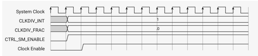
In general, an integer clock divisor of  $n$  will cause the state machine to run 1 cycle in every  $n$ , giving an effective clock speed of  $f_{sys} / n$ .
