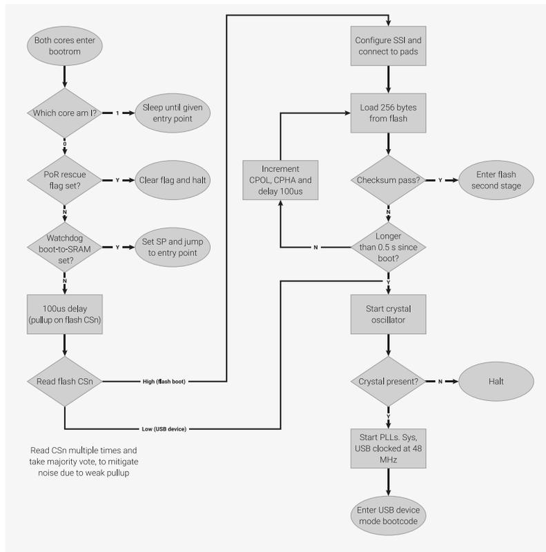
After the hardware controlled boot sequence described in [Section 2.7](#), the processor controlled boot sequence starts:
