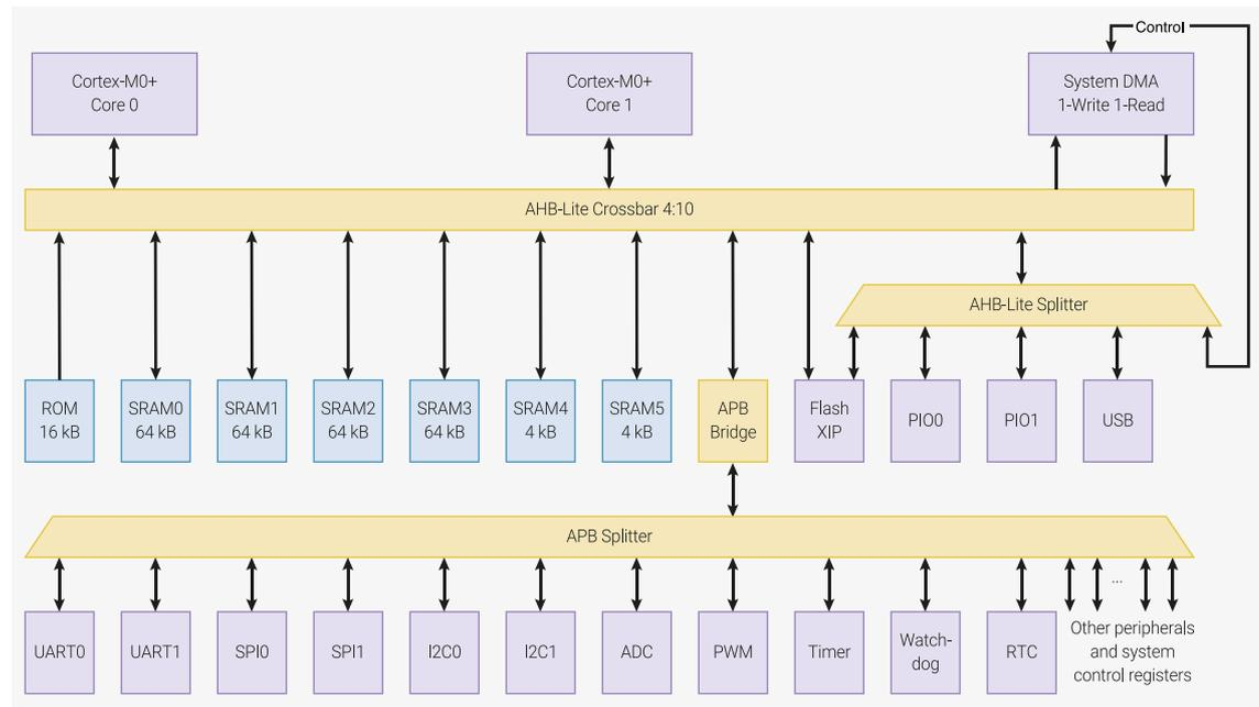
The bus fabric connects 4 AHB-Lite masters, i.e. devices which generate addresses:
