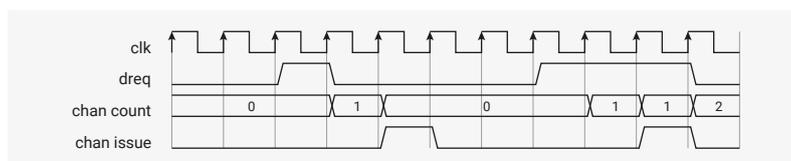
The effect is to upper bound the number of in-flight transfers based on the amount of room or data available in the peripheral FIFO. In the steady state, this gives maximum throughput, but can’t underflow or underflow.
