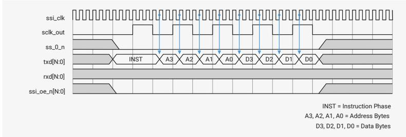
Figure 162. Transmit Data With DDR\_DRIVE\_EDGE = 2
