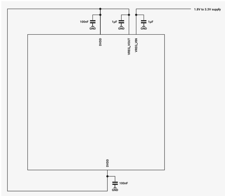
The regulator must have 1µF capacitors placed close to its input (VREG\_VIN) and output (VREG\_VOUT) pins.
