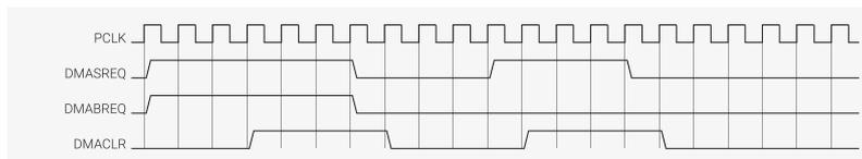
[Figure 63](#) shows the timing diagram for both a single transfer request and a burst transfer request with the appropriate DMACLR signal. The signals are all synchronous to PCLK. For the sake of clarity it is assumed that there is no synchronization of the request signals in the DMA controller.
