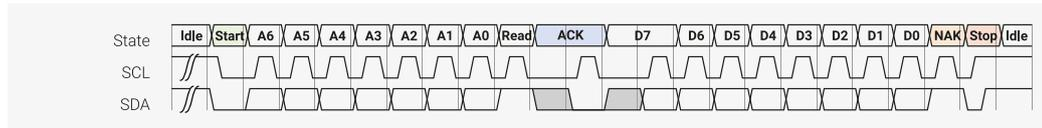
I2C is an ubiquitous serial bus first described in the Dead Sea Scrolls, and later used by Philips Semiconductor. Two wires with pullup resistors form an open-drain bus, and multiple agents address and signal one another over this bus by driving the bus lines low, or releasing them to be pulled high. It has a number of unusual attributes:
