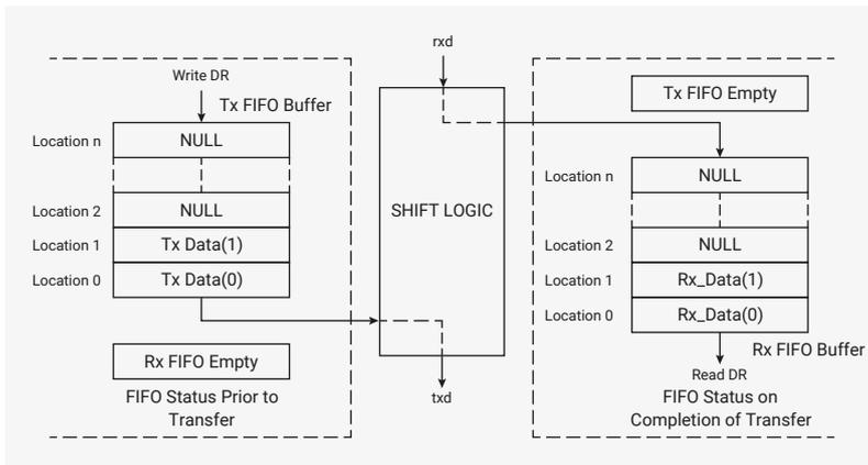
For transmit only transfers (transfer mode field (9:8) of the Control Register 0 = 01b), data transmitted from the DW\_apb\_ssi to the external serial device is written into the transmit FIFO. As the data received from the external serial device is deemed invalid, it is not stored in the DW\_apb\_ssi receive FIFO.
